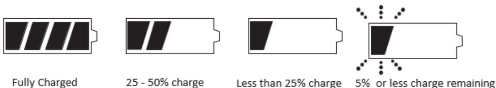
When the battery level drops to 0%, three beeps will sound and shut down.
